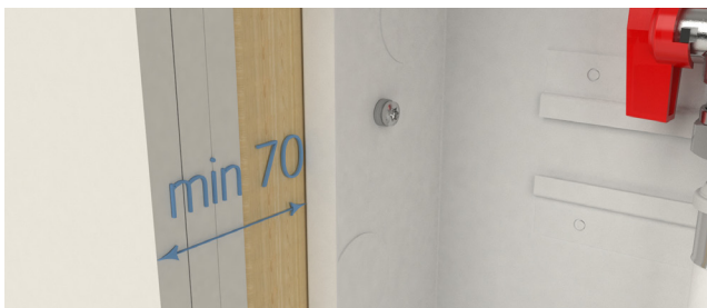
At least 70 mm from the outside plaster to the front edge of the cabinet.
